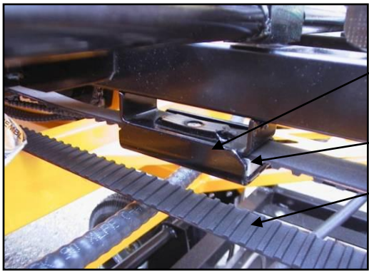
Belt Attachment Clamp Detail
